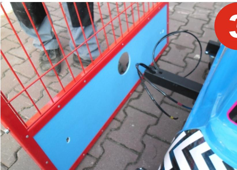
Place the front panel to the machine. Arm base must pass through the hole in the panel.
