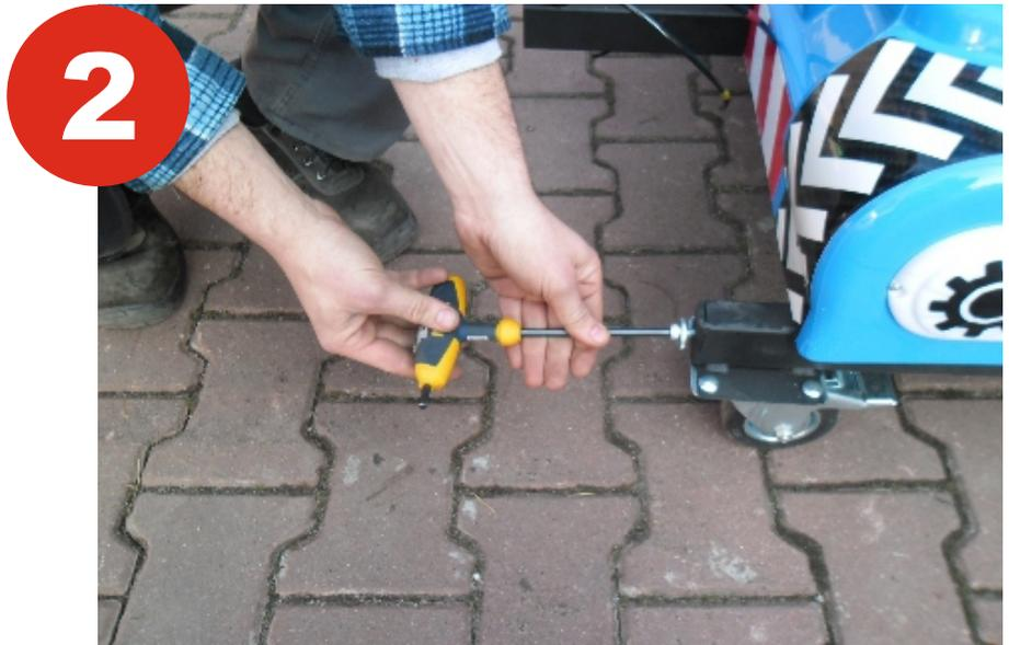
Remove the screws from the lower front part of the bulldozer
